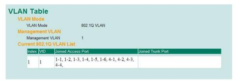
In 802.1Q VLAN table, you can review the VLAN groups that were created, Joined Access Ports, and Trunk Ports, and in Port-based VLAN table, you can review the VLAN group and Joined port.
